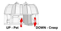
Remove detector assembly as described in Step 1. When selector is UP, Pet Mode; when DOWN, Creep Zone is active and there is no Pet Immunity. Above 2.4m Pet Immune should be OFF (lever down Pet OFF, see installation height note\*.
